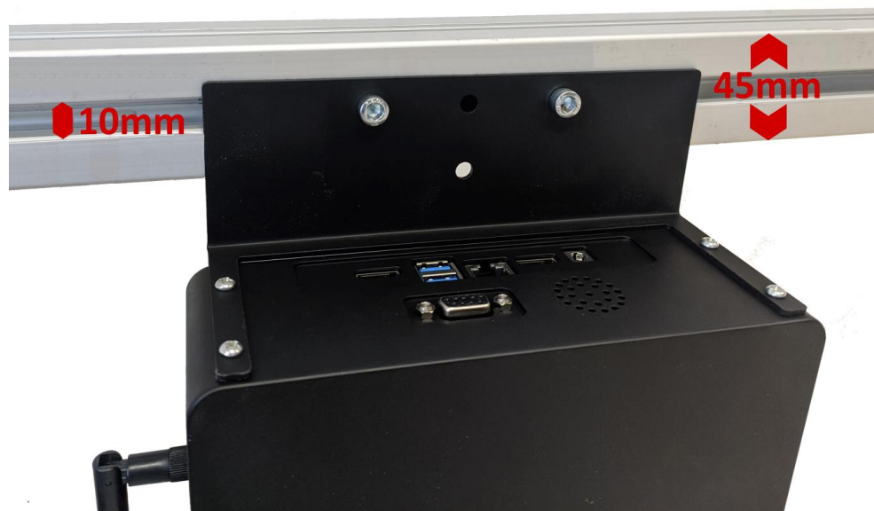
FIGURE 3: BEEVISION 270 MOUNTED ON SIGMA PROFILES
